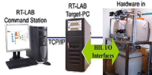
Fig. 1 Single target node
