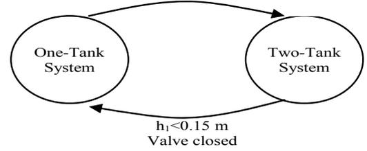
Fig. 4 Hybrid automaton of two-tank system
