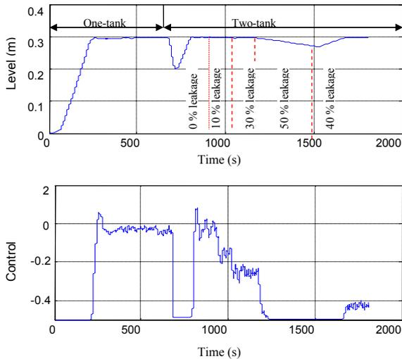
Fig. 6 Level response using adapted PID parameter
