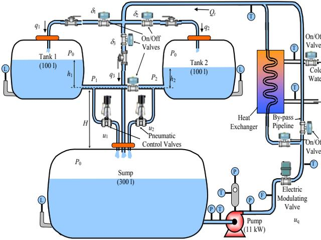
Fig. 3 Schematic diagram of two tank system
