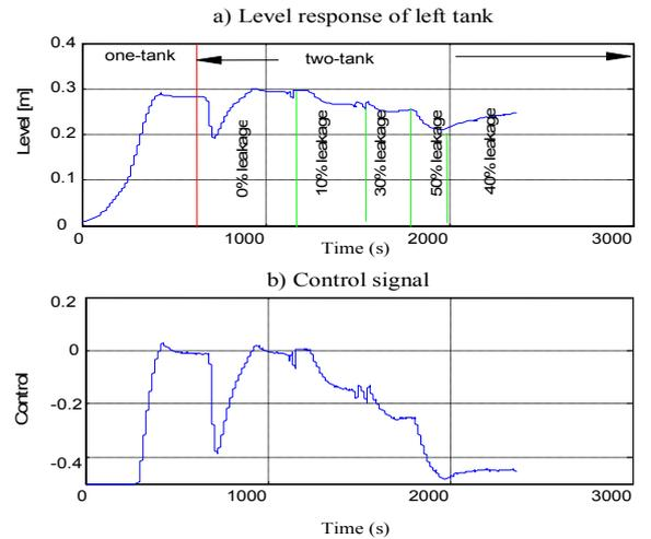
Fig. 5 Level responses using fixed PID parameters
