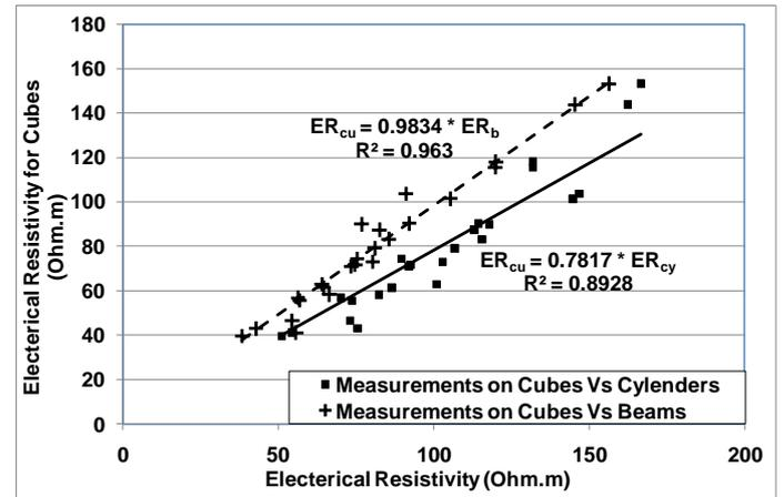
Figure 14. Relationship between electrical resistance measurements for cubes and electrical resistance measurements for cylinders and beams at different ages and water-to-cement ratios
