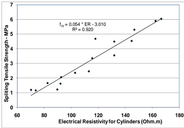
Figure 12. Relationship between splitting tensile strength and electrical resistance for cylinders at different ages and water-to-cement ratios
