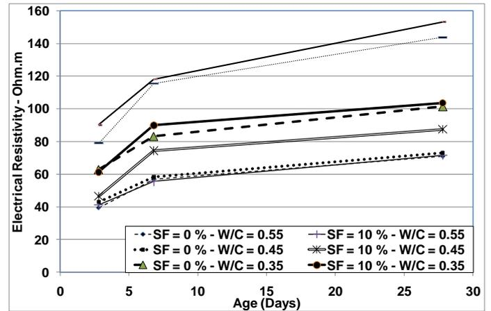
Figure 8. Effect of age on electrical resistance for cubes made with different water-to-cement ratio
