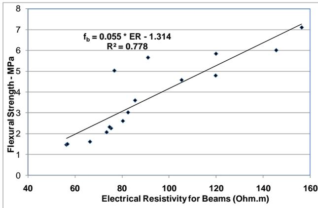
Figure 13. Relationship between flexural strength (using simple beam third-point loading) and electrical resistance for beams at different ages and water-to-cement ratios
