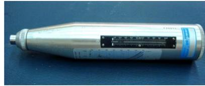
Figure 4. The used Schmidt rebound hammer tester
