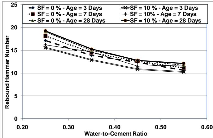
Figure 7. Effect of water-to-cement ratio on Schmidt hammer rebound number at different ages with silica fume replacement of 0 and 10 % by mass
