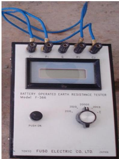
Figure 3. The earth resistance tester used
