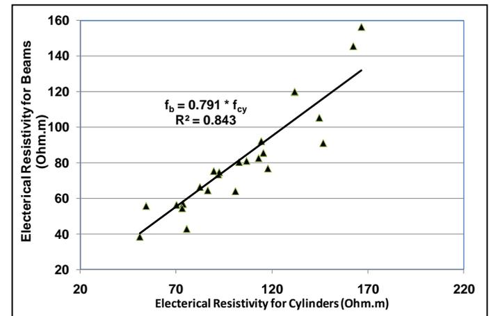
Figure 15. Relationship between electrical resistance measurements for beams and electrical resistance measurements for cylinders at different ages and water-to-cement ratios
