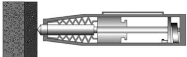
Figure 1. Schematic diagram for the Schmidt rebound hammer (ACI 228.1 R-03)
