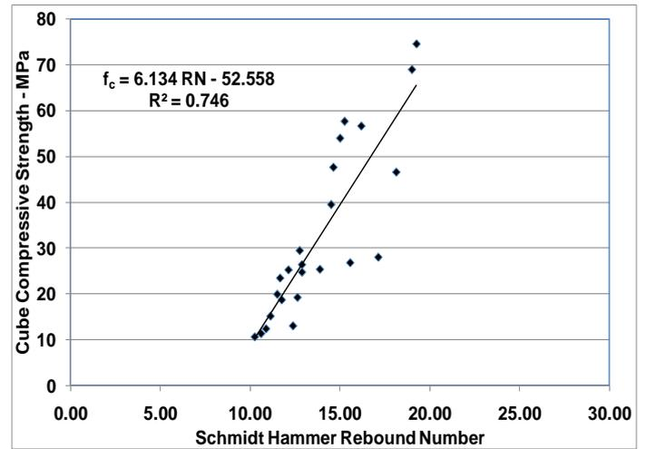
Figure 11. Relationship between cube compressive strength and Schmidt hammer rebound number for cubes at different ages and water-to-cement ratios.
