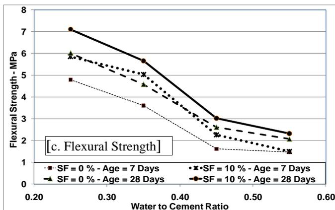
Figure 5. Effect of w/c ratio on concrete strengths (a. Cube strength - b. Splitting tensile strength - c. Flexural strength) at different ages. Silica fume replacement 0 & 10 % by mass
