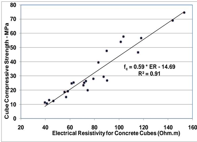
Figure 10. Relationship between cube compressive strength and electrical resistivity for cubes at different ages and water-to-cement ratios.
