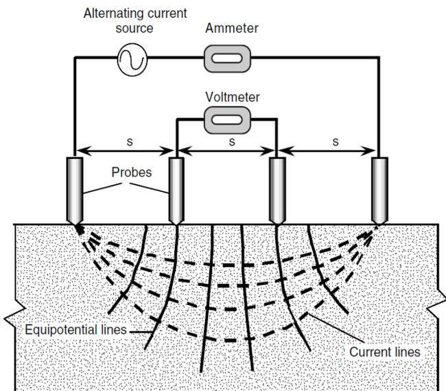
Figure 2. Four-probe resistivity test (Malhotra & Carino 2004).
