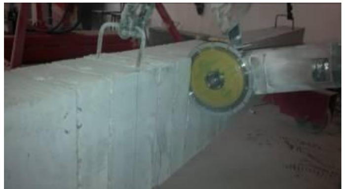
Figure 3 Cutting grooves for specimen NSM
