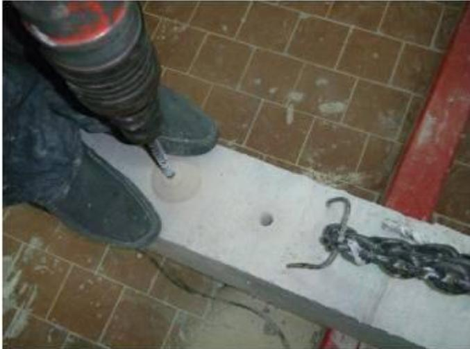
Figure 5 Drilling of holes for specimen IER-G
