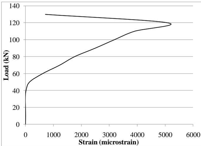
Figure 20 Strain behavior of CFRP sheet in specimen EB
