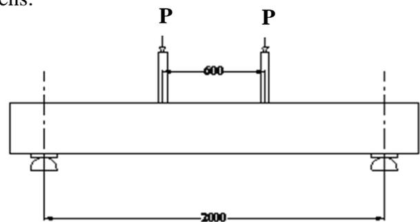
Figure 8 Test setup
