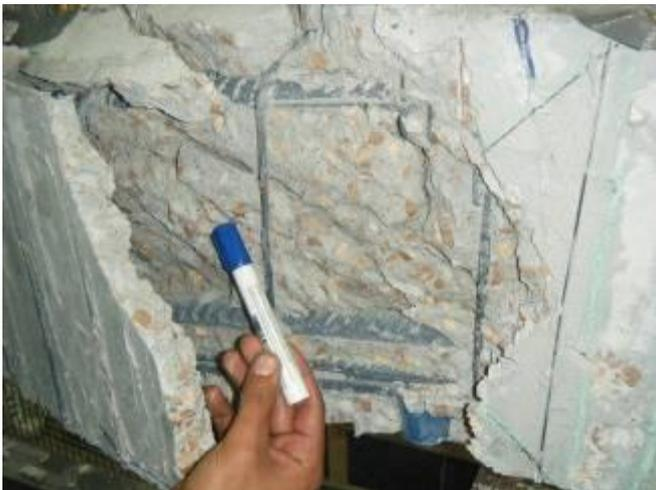
Figure 13 crack pattern of specimen NSM
