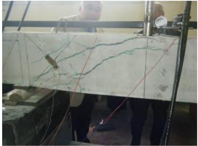
Figure 10 Crack pattern of control specimen
