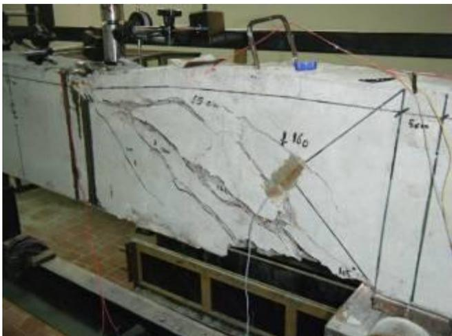
Figure 14 Crack pattern of specimen IER-G
