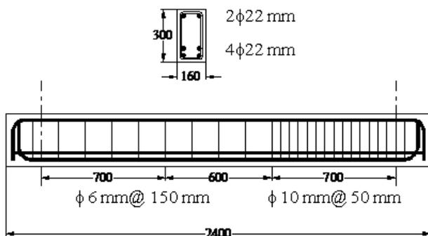
Figure 1 Reinforcement details of the specimens
