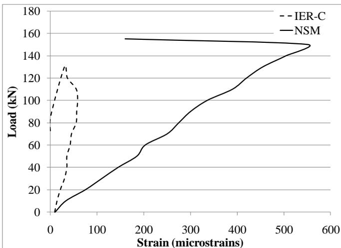
Figure 21 FRP strain behavior of specimens IER-C and NSM
