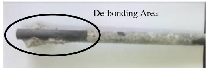
Figure 16 CFRP bar after failure of specimen IER-C
