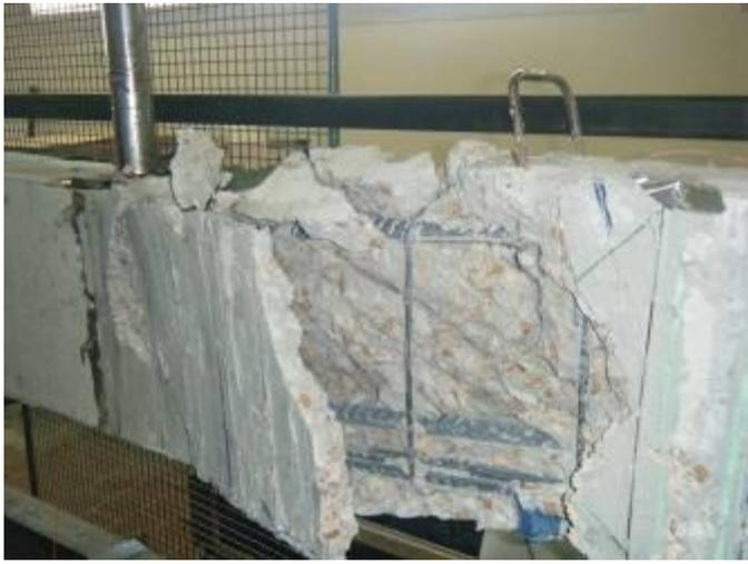
Figure 12 Failure of specimen NSM
