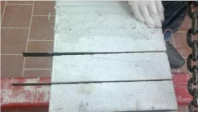
Figure 4 Installing FRP strips in specimen NSM
