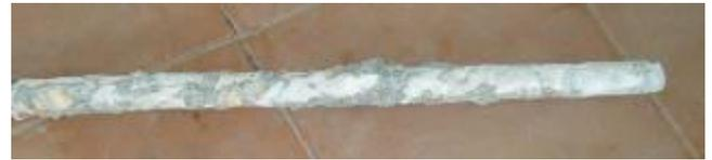
Figure 15 GFRP bar after failure of specimen IER-G
