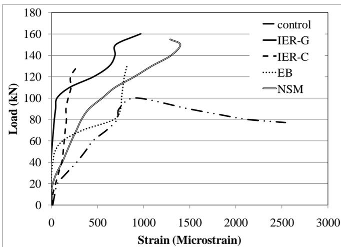
Figure 18 Steel stirrup strain behavior
