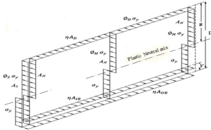
**Figure 4: Equivalent average ultimate longitudinal stress distribution over the mid-ship section of an oil tanker in damaged condition.**
